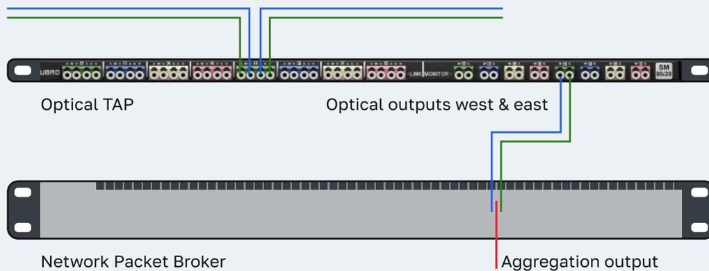
By utilizing the various filtering capabilities of the EXA48200 the user is able to further reduce traffic volume that needs to be processed, thus enabling quicker and more accurate analysis and troubleshooting. Moreover, incoming traffic can be VLAN tagged per physical port to allow easy identification at which physical port a packet original arrived.
